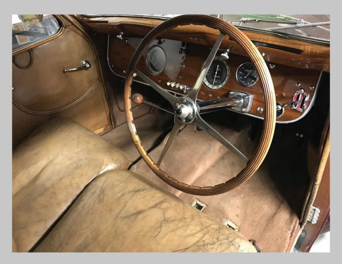
To keep the original leather properly. The seats was restored by applying new springs and reinforcing the original Leather.
